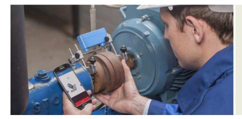
Shaft alignment is recommended for almost every industry, as it enables machine uptime to be significantly improved and maintenance costs to be reduced. The TKSA 11 focuses on industries where these shaft alignment benefits have not yet been realised and helps customers profit from correctly aligned shafts.
