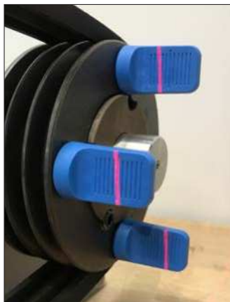
Fig.9 – Vertical angle misalignment correction
