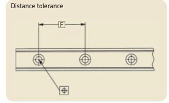
Position tolerance of rail attachment holes
